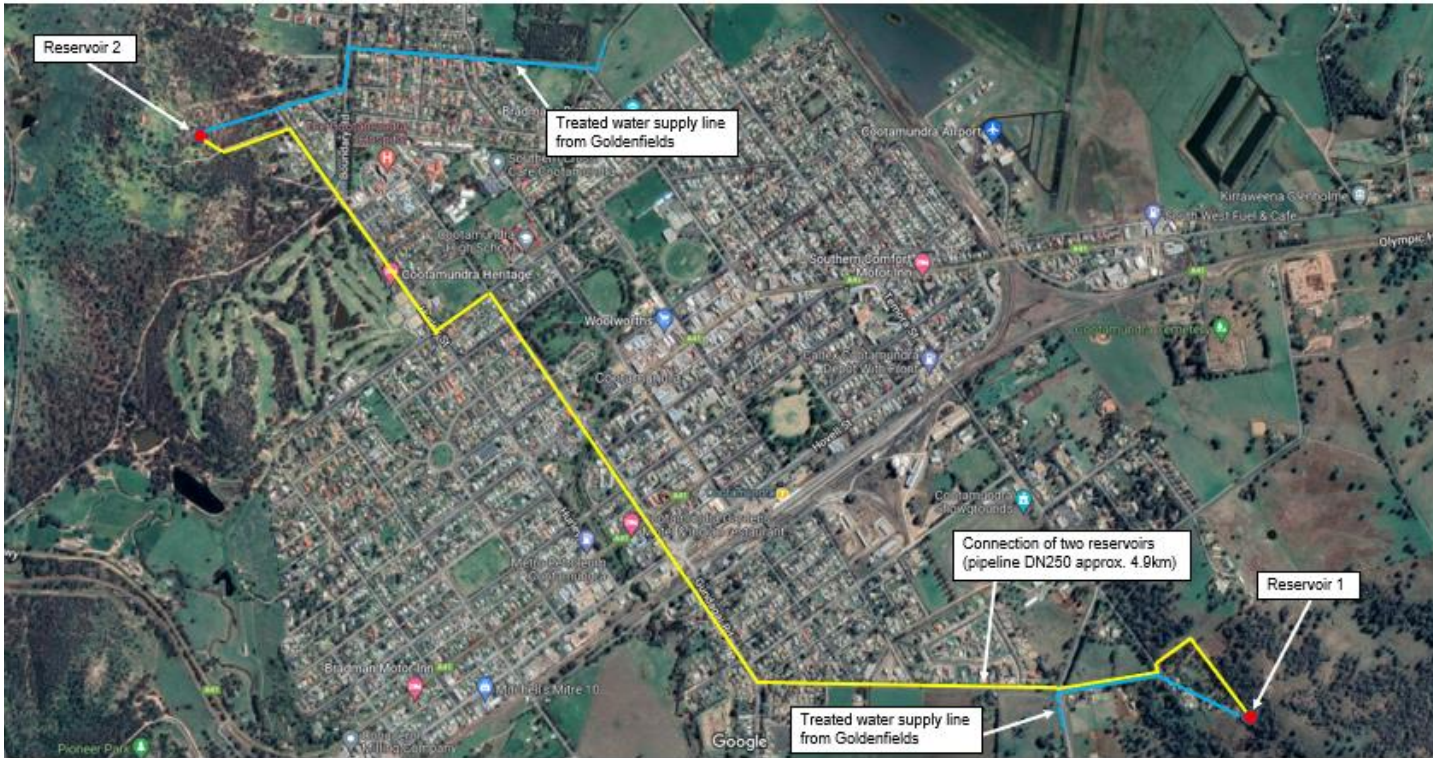
Figure 1-1: The current feed pipeline arrangement and locations of the two reservoirs
