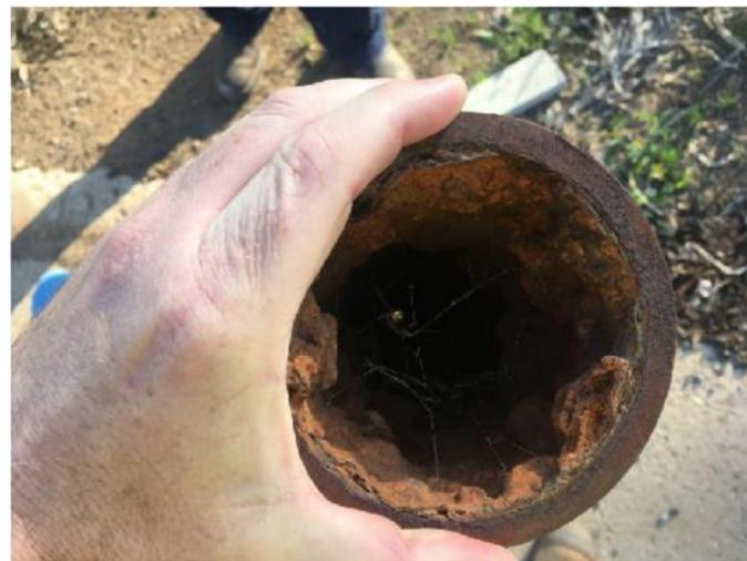
**Figure 13 Typical metallic pipe condition**
